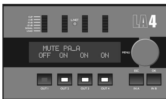
Figure 12: Output 1 is unmuted, all other 3 output channels are muted
